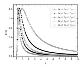
Fig. 2. LCR of ratio of Rayleigh random variable and product of two Rayleigh random variables.
