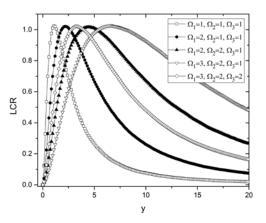
Fig. 1. LCR of ratio of product of two Rayleigh random variables and Rayleigh random variable.
