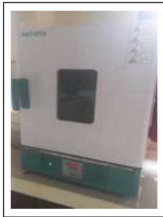
Figure 7. Heat Treatment process of ST60 steel specimens at 800°C
