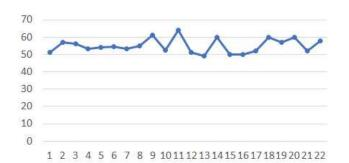
Figure 3 Graph. Hardness Value of ST37 Steel Before Heat Treatment
