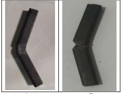
A B Figure 7.A ST37 Steel Impact Testing Results
