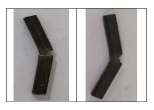
A B Figure 7.B ST37 Steel Impact Testing Results
