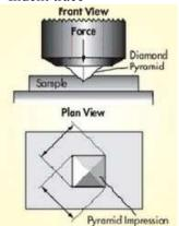
Figure 1. Vickers Hardness Testing
