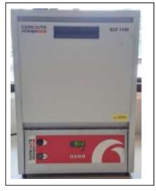
Figure 6. The heating process of ST37 steel specimens at 900°C.
