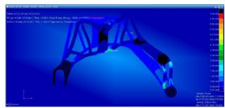
Figure 6: Strain energy (without ROD) – mode 2
