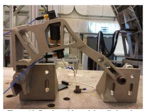
Figure 19: Bracket with stack installed on the shaker; in correspondence of the piezoceramic, two accelerometers are visible
