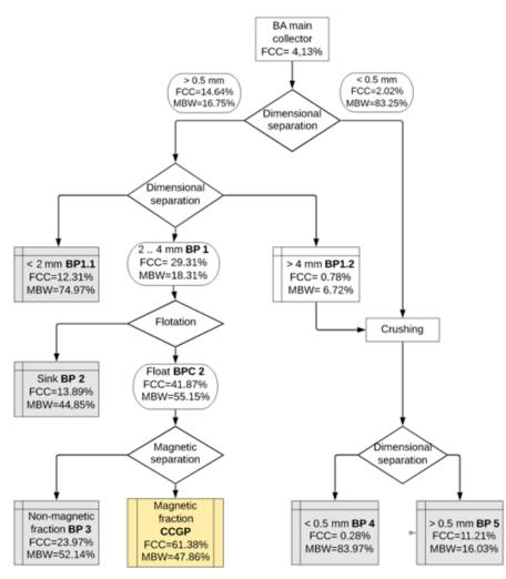
Figure 2. Overall process flow for complete BA recycling
