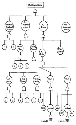
Fig.3 Fault tree diagram of the reverse osmosis plant.
