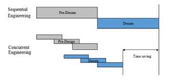
Figure 2: Sequential engineering vs. concurrent engineering [7].
