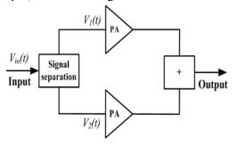
Figure 3: Linear amplification using Nonlinear Components (LINC)
