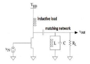
Figure 2: Sinusoidal Power amplifier
