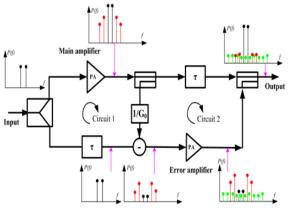
Figure 4: Feedforward Technique
