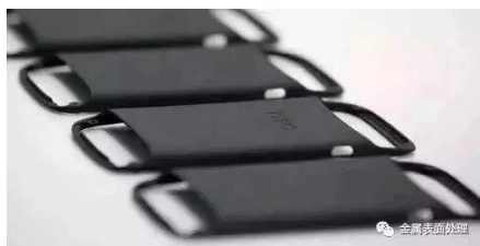
Fig. 9. Examples of details by electrophoresis and microarc oxidation [6, 7]
