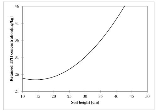
Figure 8: Retained TPH concentrations in varying soil depths.
