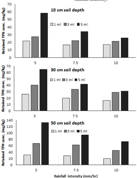
Figure 7: Retained TPH concentrations for various soil depths and rainfall intensities
