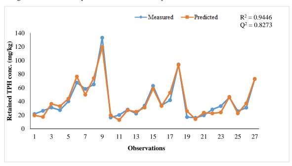
Figure 12: Comparison of measured and predicted retained TPH concentrations with different observation points.
