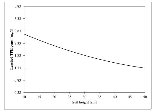
Figure 2: Leached TPH concentrations through varying soil depths.
