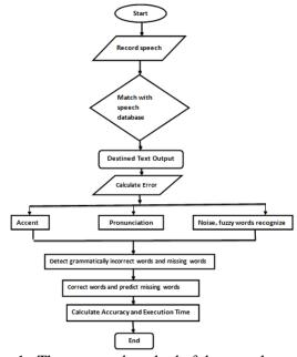
Figure 1. The proposed method of the speech recognition system
