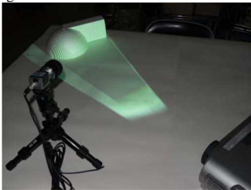
Fig.4 System setting for multiple structured lights projection.
