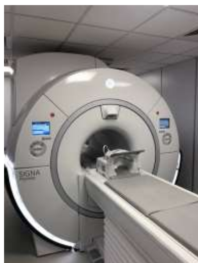
Figure 1. The equipment used in this study - 3.0 T Signa Pioneer MRI scanner produced by GE Healthcare
