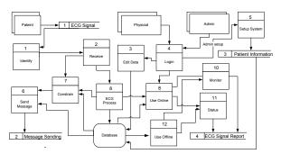
Figure 8. The Data Flow Diagram of ECG signal processing application
