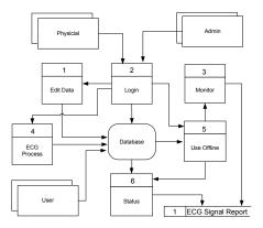
Figure 11. Data Flow Diagram of web services over WBBNS and the internet
