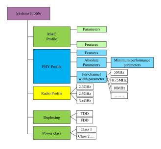
Figure 2 Structure of fixed and mobile WBBNS system profile.
