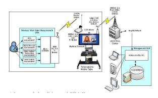
Figure 4. Structure of telemedicine via Wi-MAX
