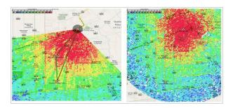
Figure 16. Radiation pattern of 3-sectors antenna system, the distance between the MSMC to two health sub-district
