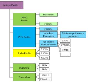
Figure 2 Structure of Fixed and Mobile WiMAX system profile.
