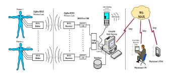
Figure 6. The structure of the signal processing system in the ECG monitoring
