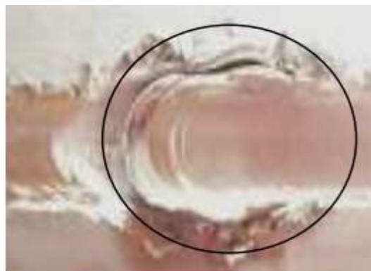
Figure 3.(b) AZ alloy produced with a pin type probe
