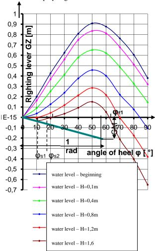
Fig. 4. Influence of the amount of water in the compartment on the Reed's curve
