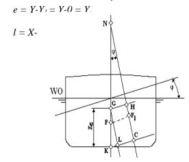
Fig. 3. Righting lever of the shape and mass [1]
