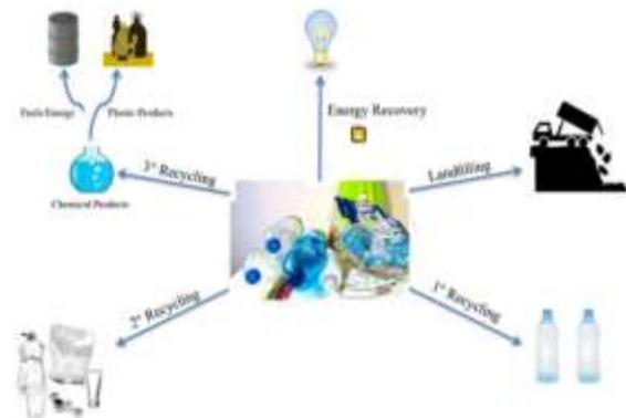
Fig. 1. Different methods of recycling plastic waste.
