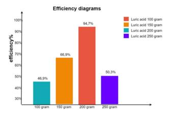
Figure 13. Cooler box efficiency with PCM lauric acid and ice pack.
