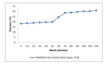
Figure 7. Cooler box graph without PCM.
