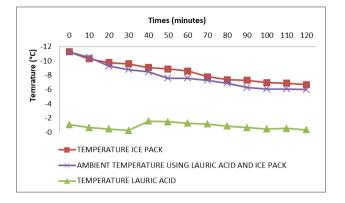
Figure 9. Cooler box graph using 250 gram lauric acid and ice pack as control
