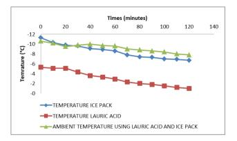
Figure 10. Cooler box graph using 200 gram lauric acid and ice pack as control
