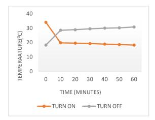
Figure 6. Graph temperature vs times peltier in cooler box
