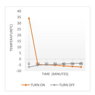
Figure 8. Graph of temperature vs times with ice packs containing frozen food in cooler boxes.
