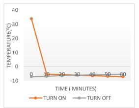
Figure 7. Graph of temperature vs times with ice packs in cooler boxes.
