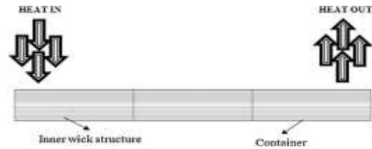
Fig. 2 Schematic of a tubular heat pipe.
