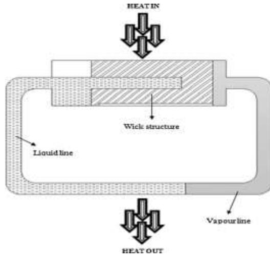
**Fig. 4.** Schematic of a loop heat pipe arrangement.
