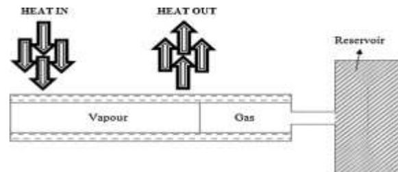
Fig. 3. Schematic of a cold-reservoir variable conductance heat pipe.
