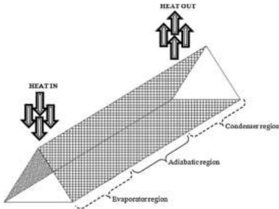
**Fig. 5.** Schematic of a micro heat pipe.
