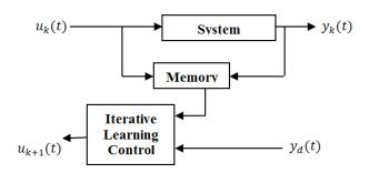
Fig. 4. Basic block diagram of the ILC system
