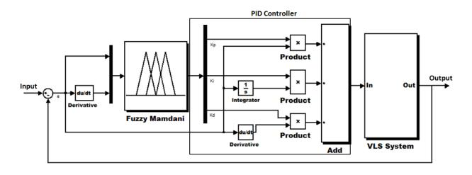
Fig. 3. Block diagram of VLS control system by using Fuzzy PID controller
