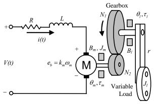
Fig. 1. Equivalent circuit of the VLS system
