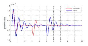
**Fig.4** functioning system in the nominal régime used of TBB-500 connected to a long line with,  $H\infty$  -PSS,PSSPID(robustness tests) (Ug, Pe ,glissement
