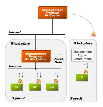
Fig. 1 The overview of oyster output management system
