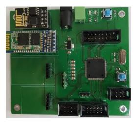
Fig. 10 Developed PCB of the embedded system
